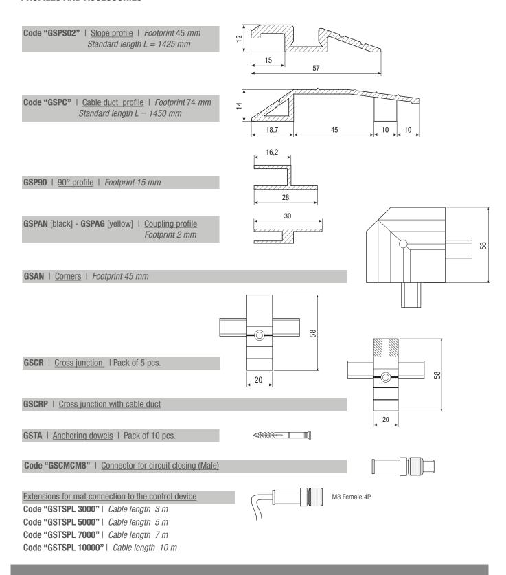
Example: Modular safety mat with dimensions 1000x1500 mm (profile type "GSPS02") maximum footprint 1090x1590 mm.
