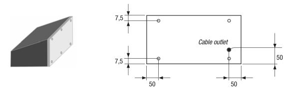
**Type "C"** Frame-plate flush with the bumper and with M6 stud bolts, 30 mm long, for fastening to the inside of the machine via bolts.
