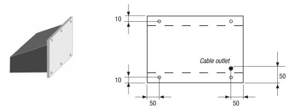
**Type "B"** Frame-plate flush with the bumper and with threaded holes (specify when ordering) for fastening to the inside of the machine via screws.
