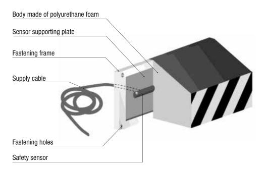
The bumper is equipped with a 4-pole outlet cable, 4x0.35mm2 FROR 300/500 – standard length 3 m.
