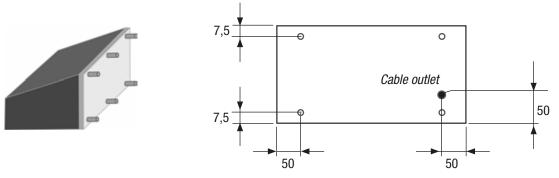
N.B. For bumpers longer than 500 mm, other additional fastening holes will be drilled (centre distance from one hole and another  $\leq$  500 mm.
